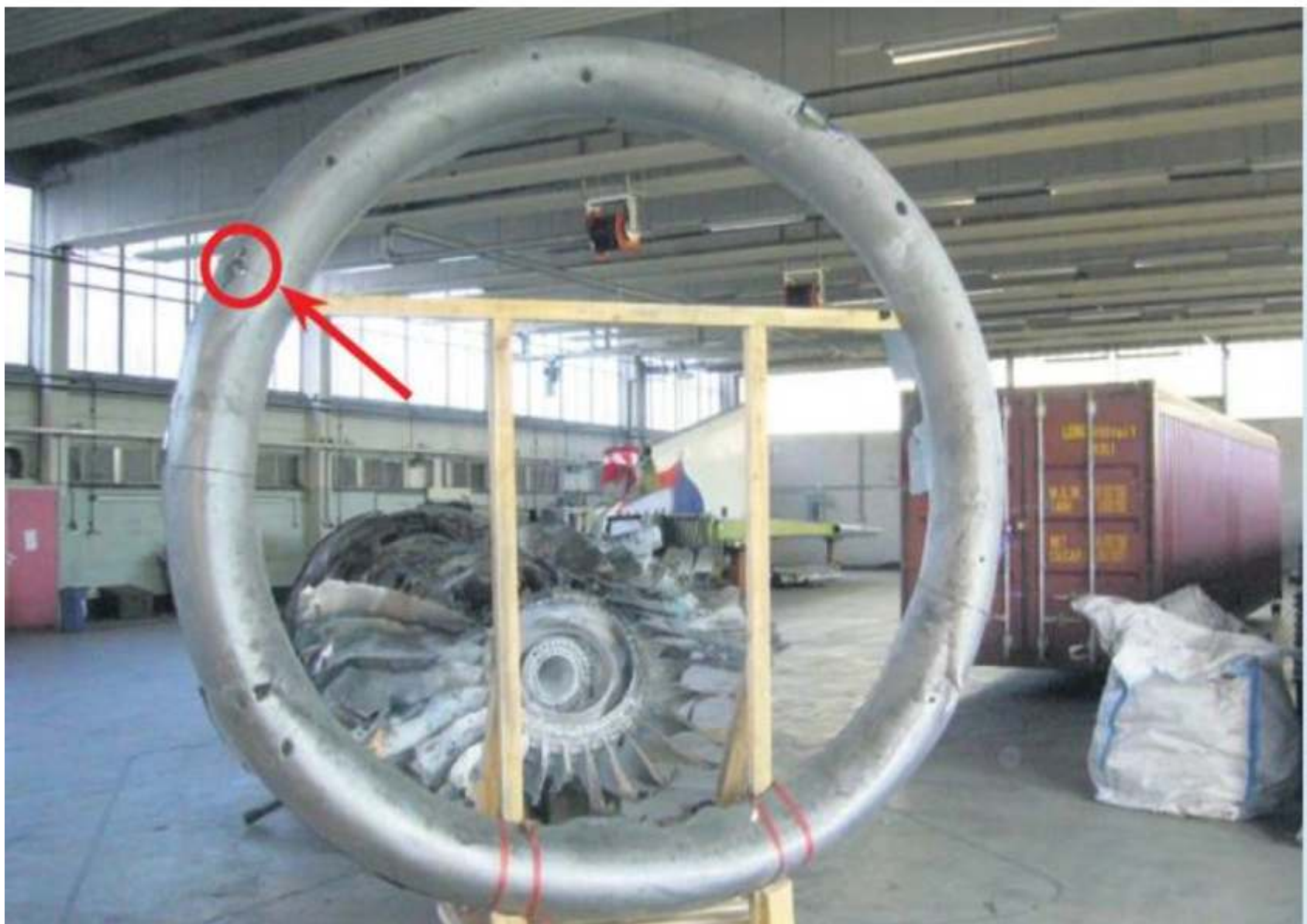
Left engine inlet ring damage analysis
