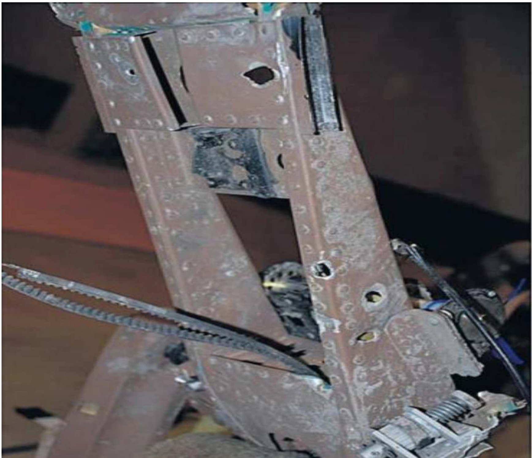
Damage patterns inconsistent with Buk missile fragmentation
