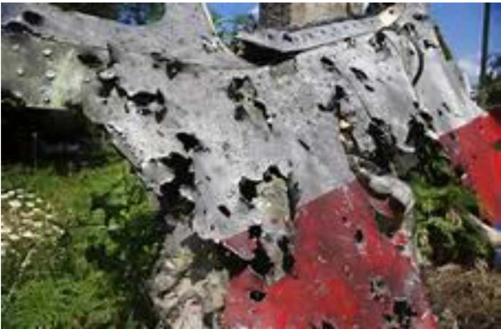
Buk-particle impacts or 30mm bullet impacts?
